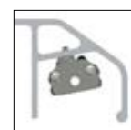
Fix orientation of luminaire with two screws (one in each end)
