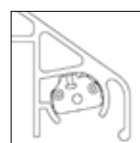
Fix orientation of luminaire with two screws (one in each end)
